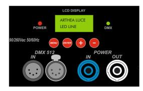
Connect the provided XLR cable to the female 5-pin XLR output of your controller and the other side to the male 5-pin XLR input of the moving head. You can chain multiple projectors together through serial linking. The cable needed should be two core, screened cable with XLR input and output connectors. Please refer to the diagram below. DMX-512 connection with DMX terminator.
