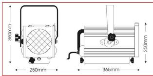
Quality 1/1200W pc spotlight with a screw focus variable-spread tight-edged beam, an easily adjustable lamp position for either 1000W or 1200W lamps, effective tilt lock and double-microswitch interlock for safe lamp replacement.
