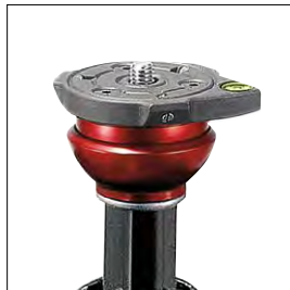
Center column with built-in 50mm half ball locked using the rotating grip located at the bottom of the center column. Tilt range: +15^{\circ}/-15^{\circ} .
