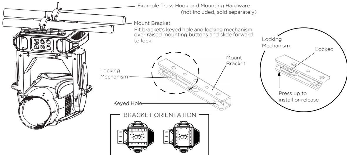
**Installing in Truss:**
