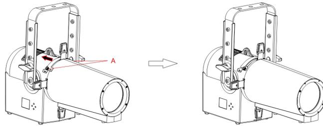
Step 2. Snap the iris into the luminaire as shown.
