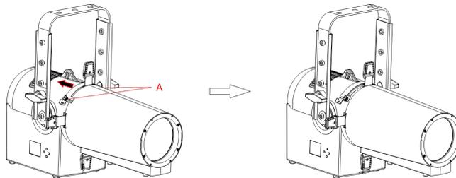
Step 2. Snap the gobo holder into the luminaire.
